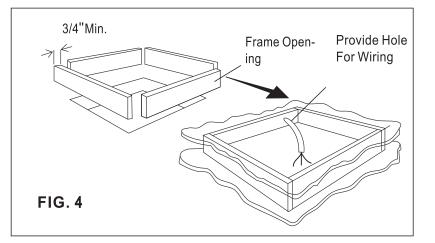
5. The 14-1/4" x14-1/4"(<u>+</u>1/8) roof opening is part of the return air duct and must be finished in accordance with NFPA standard 501C, Standard for Recreational Vehicles, Section 2-7.
